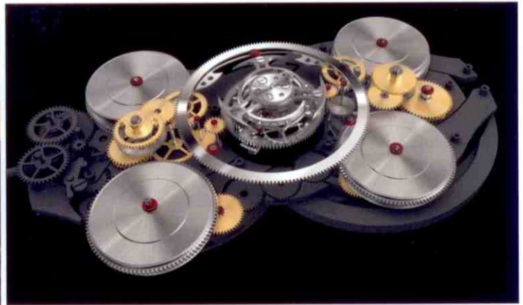
The hour and minute hands have to communicate with each other across the massive divide between them. This was accomplished with an oversized, ultra-flat, mirror-polished wheel centrally located under the dial
