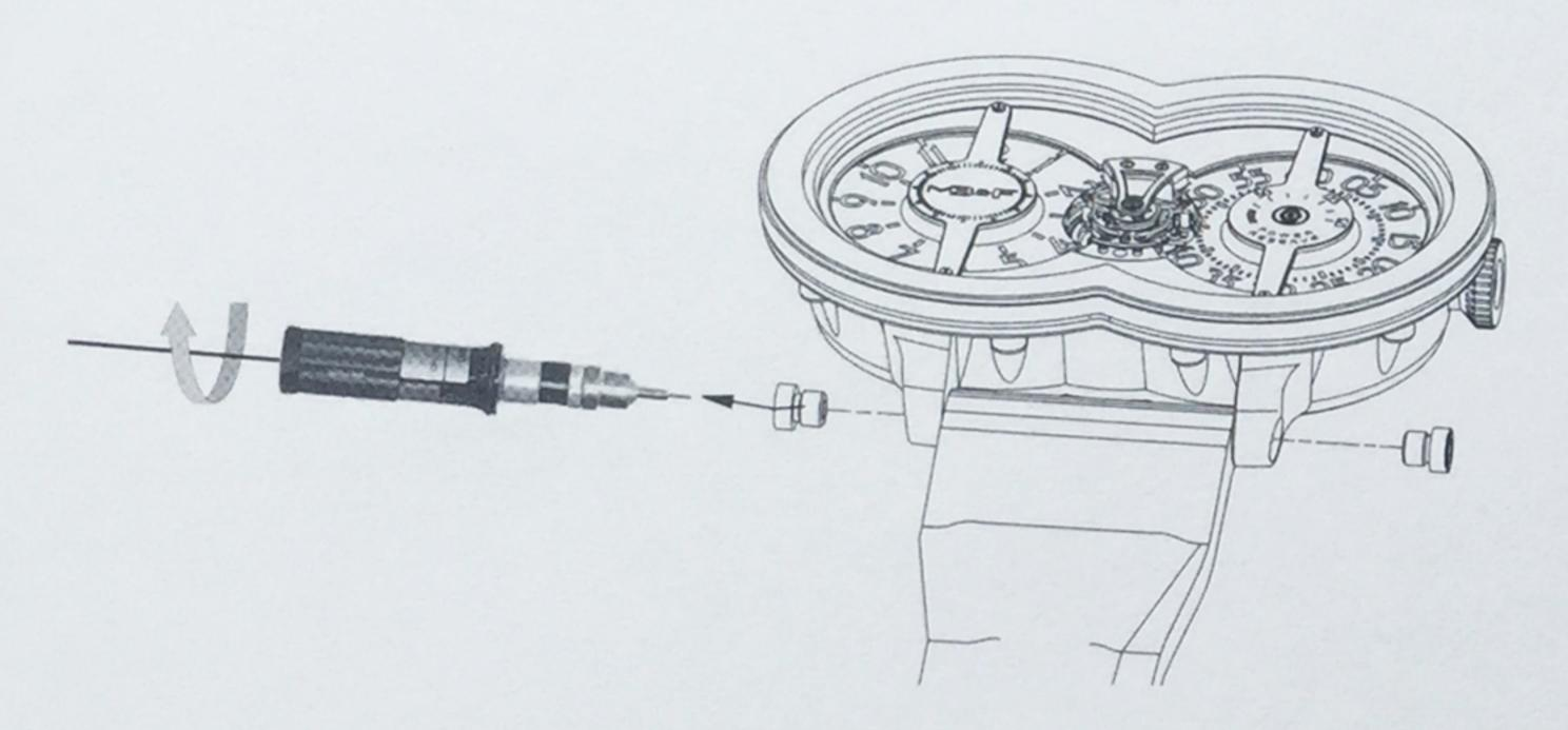
2. Remove the screw on the left-hand lug by turning anticlockwise with the supplied dynamometric screwdriver.
