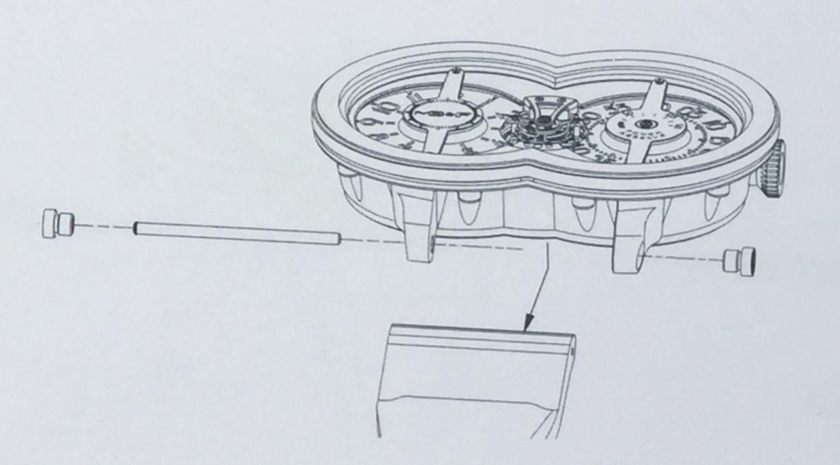
3. Push the central pin out from between the strap and the lugs and remove the strap. Repeat steps 1-3 on the other side of the case.
