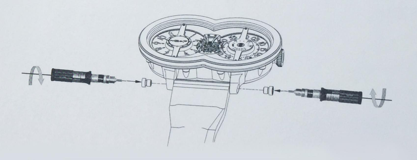
5. Screw-in the left and right-hand screws into the lugs by turning the dynamometric screwdriver in a clockwise direction. Take care not to force or over-tighten screws. Repeat steps 4-5 on the other side of the case.
