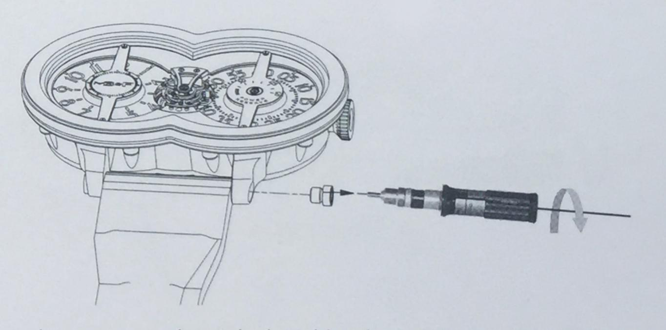
1. Remove the screw on the right-hand lug by turning anticlockwise with the supplied dynamometric screwdriver.
