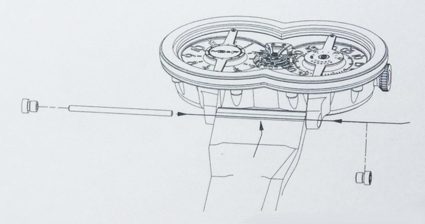
4. Place the new strap between the lugs and slide the central pin through lugs and strap.
